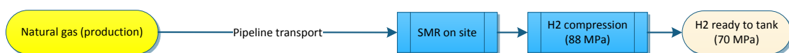
Figure 1 - H 2 production route 1: H 2 production by SMR on-site with an input of natural gas.
